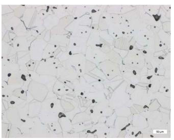
Predominately austenitic structures with rounded pores and minor fraction of delta-ferrite.
