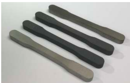
Specimens with subsequent process steps, bottom to top: as sintered, after hardening, after tempering and after blasting.
