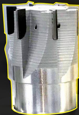
Guhring UK has sent metal 3D printed tools to customers to test new concepts.
