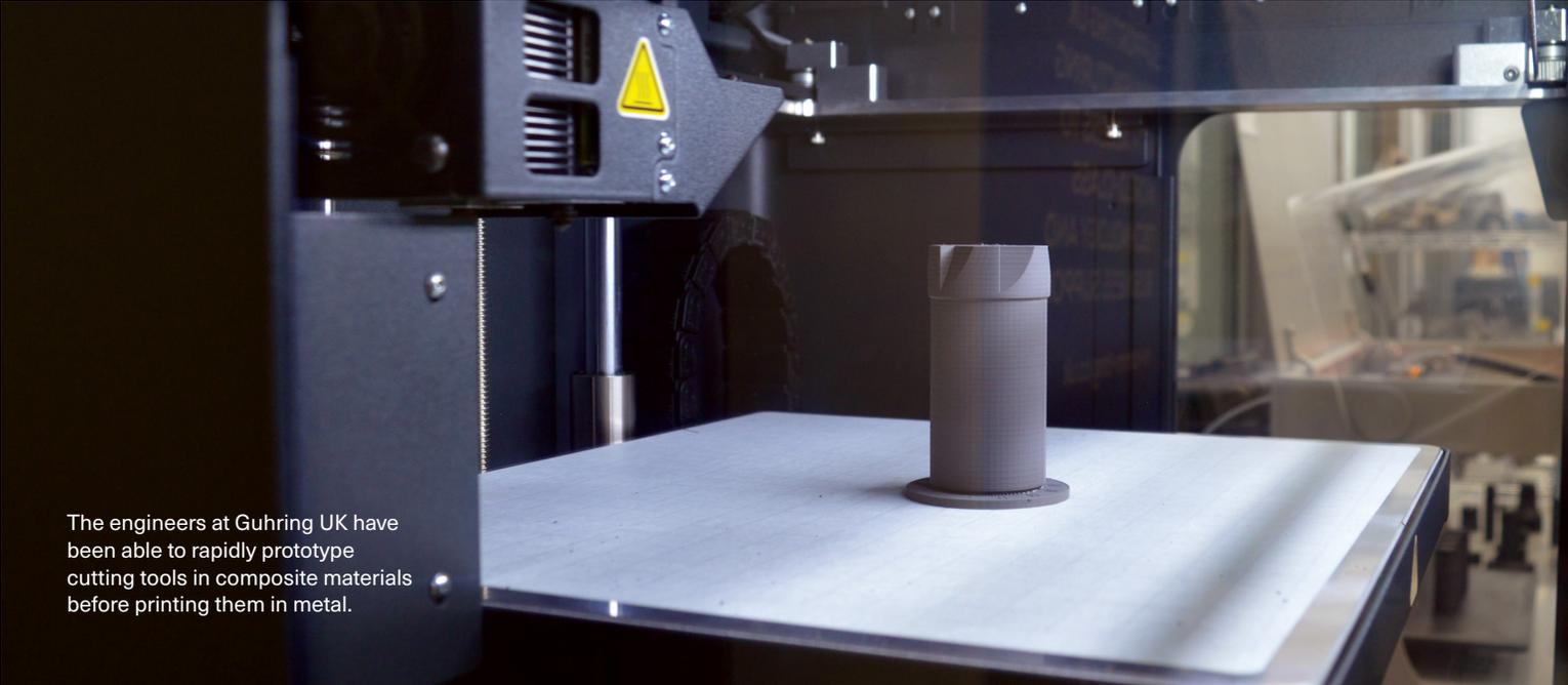
The engineers at Guhring UK have been able to rapidly prototype cutting tools in composite materials before printing them in metal.
