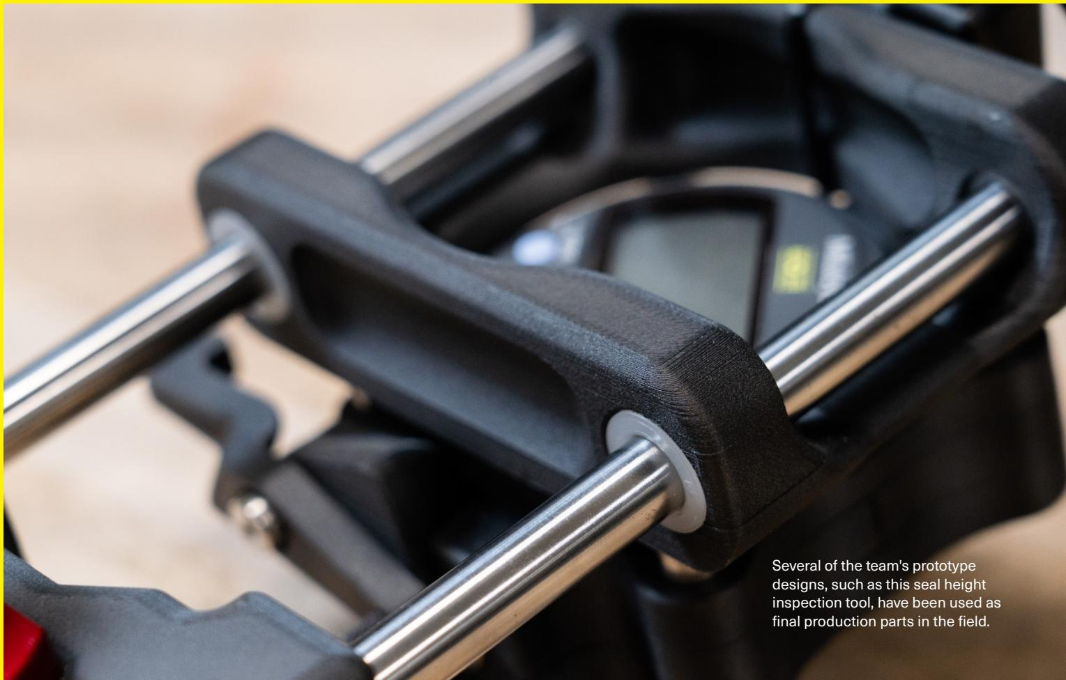
Several of the team's prototype designs, such as this seal height inspection tool, have been used as final production parts in the field.
